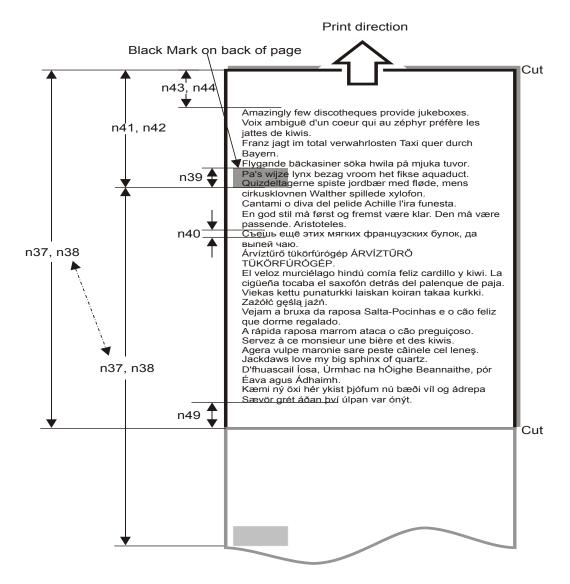
Top margin, bottom margin, page length, and synchronization with preprint are set up with parameters in the printer.
